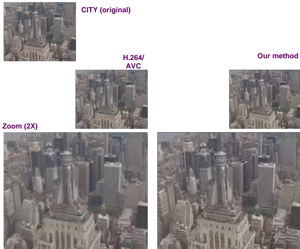
Figure 7. Coding results for a frame of CITY at QCIF resolution, 15Hz, 64kbps.
